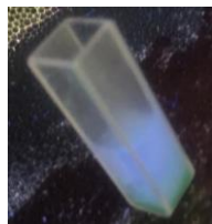
Figure 25: Fluorescence of the last sample of reaction at 135 min under the UV lamp.
