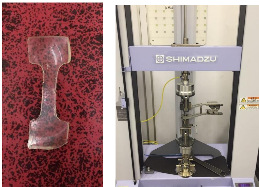
Figure 20. Equipment employed to mechanical test and the proper cut sample (model AGS-X-Shimadzu).
