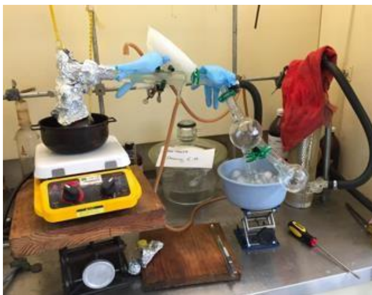
Figure 12. Assembly for distillation of AAc under reduced pressure
