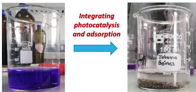
Figure 11: CV dye in solution and Discoloration by SXQ-102 after 2 hours.
