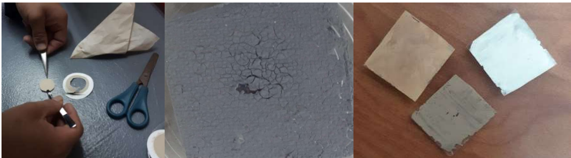
Figure 3.21 Methods offered by Hauff et al (1984) and Moore & Reynolds (1989). A) Filter was cut to fit in the sample holder B) Sample adopted the roughly surface of the filter. C) Transfer method samples.
