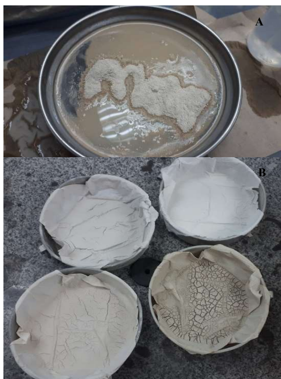
Figure 3.4: CELEC's procedure. A) Water for screening B) Material after heating at 60°C.
