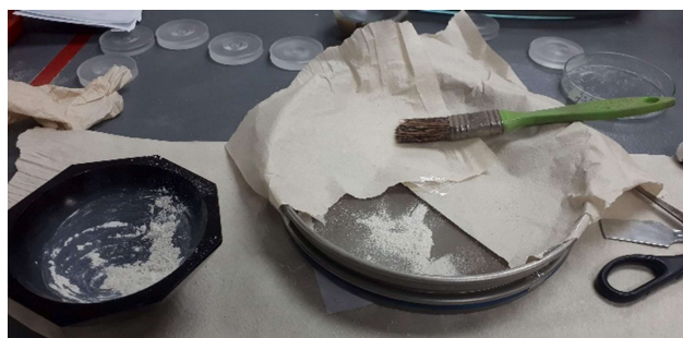
Figure 3.5: Sieving of the material without water, only using a brush and agate mortar.
