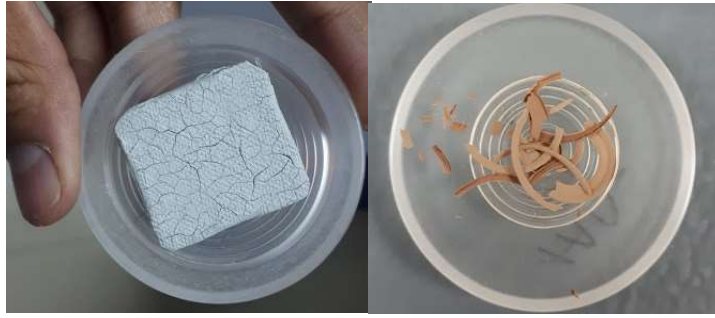
Figure 3.20 Damage in the sample either cracks or curls.
