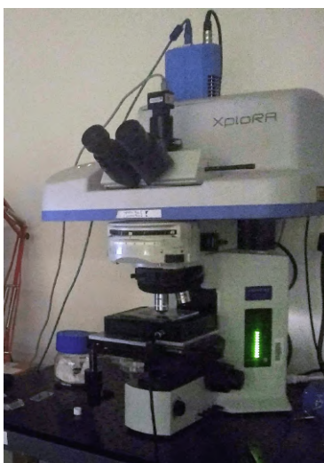
Figure 4.7: Raman XPLORA equipment belonging to the Freie Universitat Berlin (FU), Germany.
