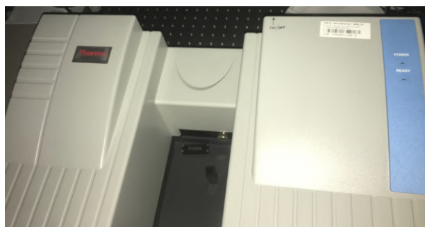
Figure 4.8: UV-visible spectrophotometer by Thermo Fisher Scientific equipment belonging to the Freie Universitat Berlin (FU), Germany.
