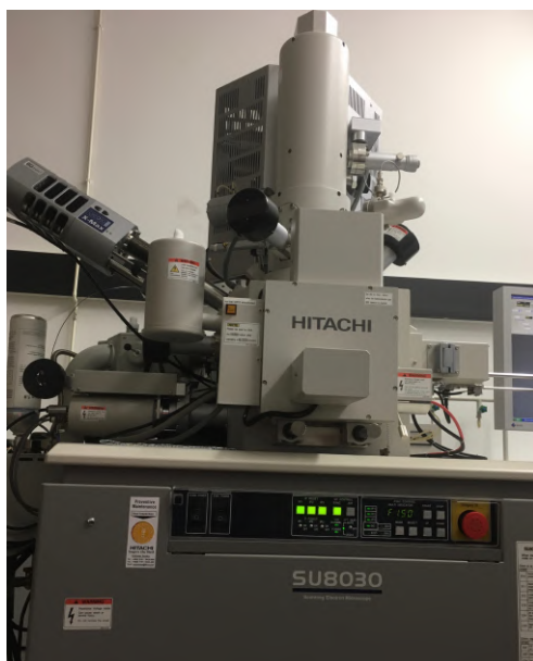
Figure 4.5: Scanning electron microscopy Hitachi SU8030 belonging to the Freie Universität Berlin (FU), Germany.
