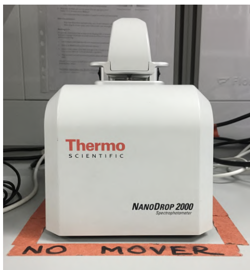
Figure 4.10: Nanodrop 2000 Thermo Scientific Spectrophotometer equipment used to measure the optic density for cell cultures, belonging to the YachayTech University, Ecuador.
