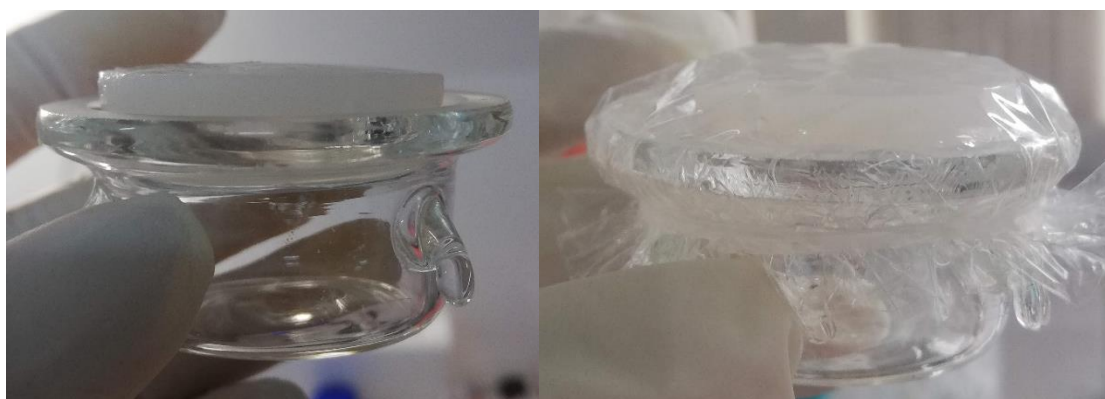
Figure 22: Assembly of the hydrogel in the donor chamber of the Franz Cell with the cellophane membrane.
