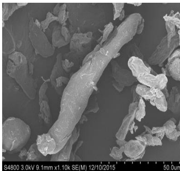
Figure 17: SEM analysis of cellulose fibers
