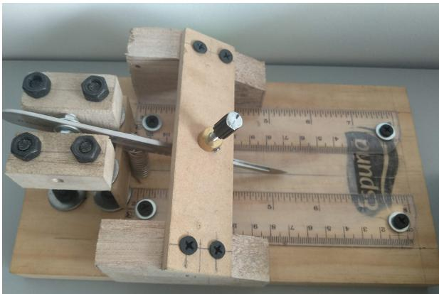
Figure 3.4: Guillotine used to cut the constriction on the gold wire. It consists of a fixed scalpel whose vertical position is adjusted using a micrometer screw. The gold wire is placed over a glass slide that can move following the ruler guides. In this way, the wire can roll under the scalpel and then it cuts a circular cross-section in the wire that forms the constriction.
