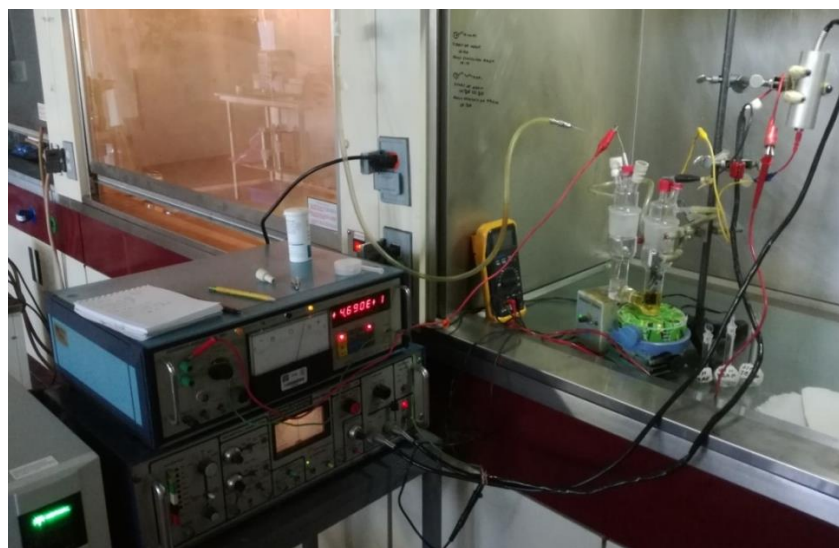
Figure 23. Setup used for electrolysis. Equipment: Power Supplier, Coulombbimeter, Potentiostat/Galvanostat, Multimeter, H-type cell and stirring devices.
