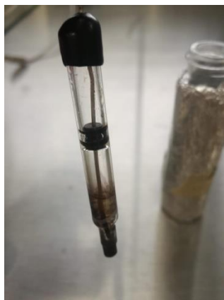
Figure 1. Ag/Ag + reference electrode used for cyclic voltammetry and electrolysis experiments.
