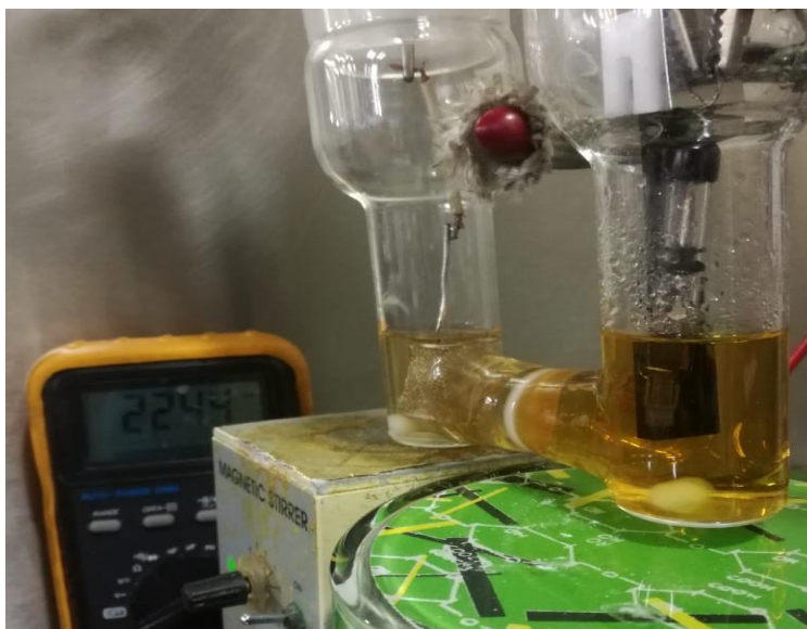
Figure 22. Close-up of the H-type divided cell during electrolysis. On the closer compartment the analyte being reduced and W.E and R.E dip in solution while adopting a deep yellow color. On the farther compartment the complementary oxidation reaction taking place on the dip C.E. and staining yellowish-clear the supporting electrolyte. Stirring was set at a moderate rate.
