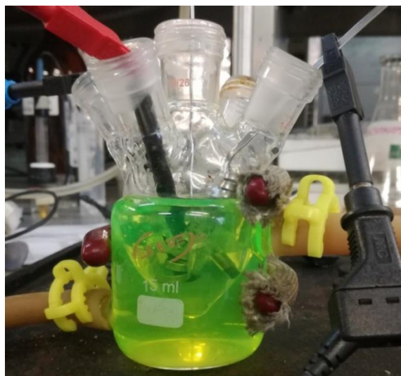
Figure 2. 15mL thermostated heart-shaped electrochemical cell used for Cyclic Voltammetry.
