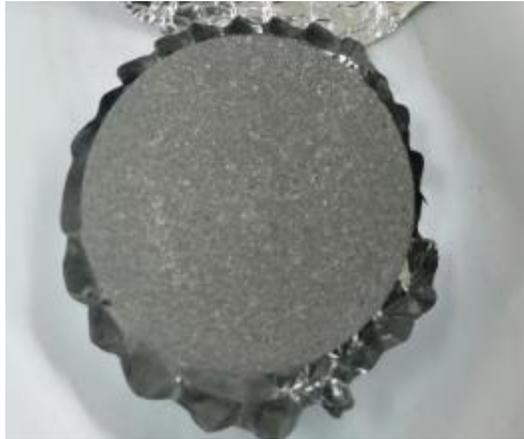
*Figure 11: Sample tablet for EDS analysis.*
