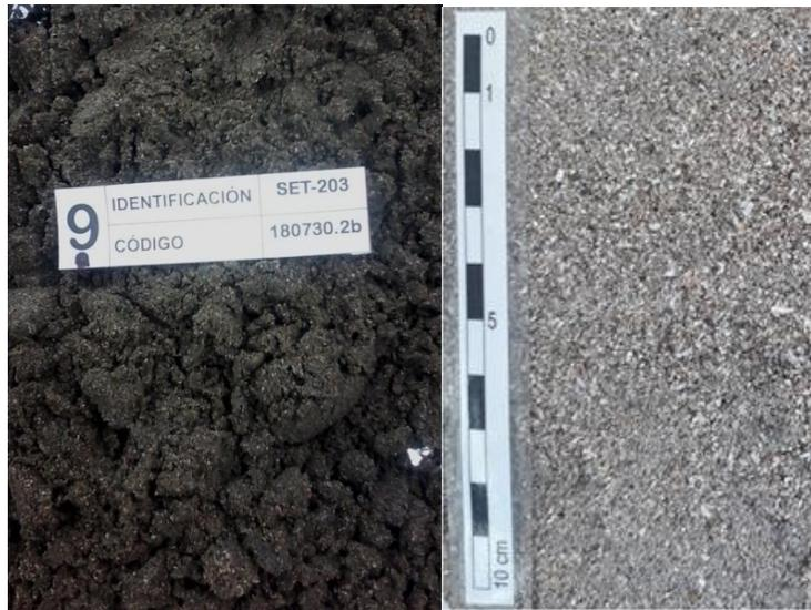
Figure 17: Comparison between wet (left) and dry (right) sand sample SET-203<sup>26</sup>.
