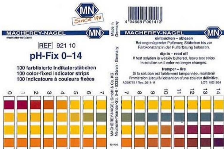
Figure 14: Macherey-Nagel 921 10 color-fixed pH indicator paper scale<sup>40</sup>.
