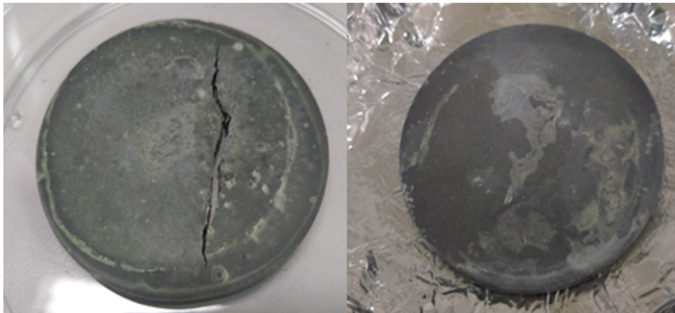
Figure 3.4: Target of \text{KNNCu}0.5\%\text{mol} (1) and \text{KNNCu}1\%\text{mol} (2), calcinated at 900^\circ\text{C} for 4 hours and sintered at 1100^\circ\text{C} for 1 hour.
