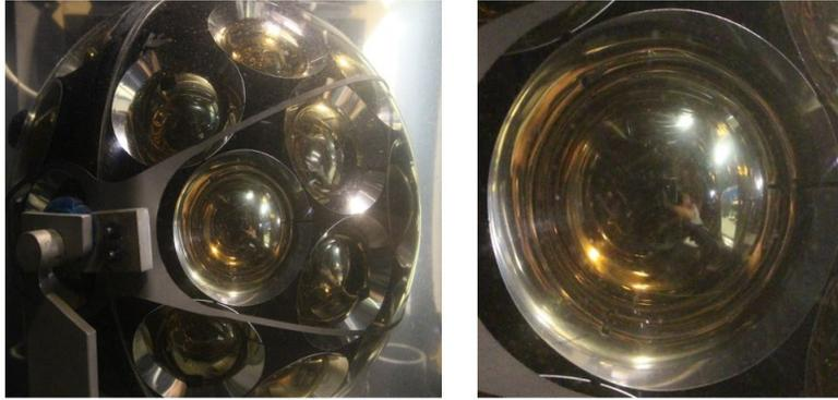
Figure 6.1: **Location of the DOM at  $180^\circ$** . Left: picture of the whole DOM inside the aquarium. Right: view from the line of sight of the laser. The angle between the laser and the optical axis is  $180^\circ$ .
