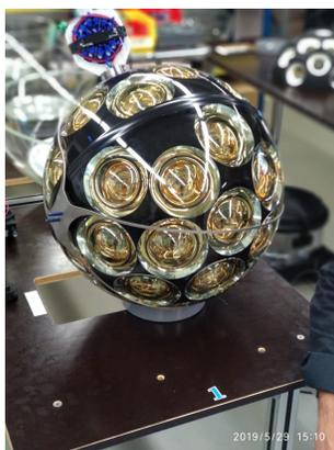
Figure 3.1: **The KM3NeT DOM.** A DOM consists of a glass spherical vessel, 31 PMTs arranged to look in all directions, LED, CLB, PB, associated readout, power supply and communication.
