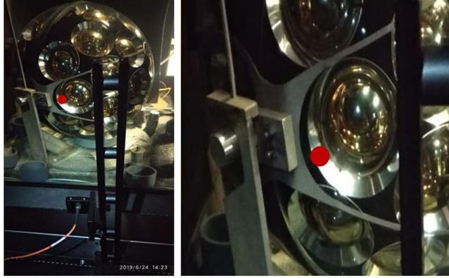
Figure 5.5: **PMT mounting frame.** Left: The PMT close to the titanium collar is marked with a red point for reference. The collimator is on the rails in front of the PMT. Right: Close view of the titanium collar and vertical support.
