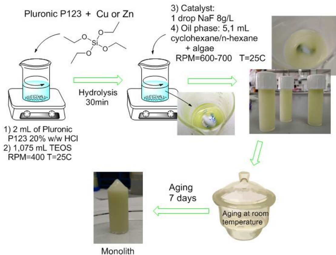
Figure 2.1 Scheme of the synthesis of algae-silica monoliths.
