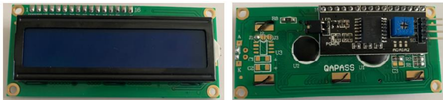
Figure 13: Right: Display. Left: Bus I2C [14].
