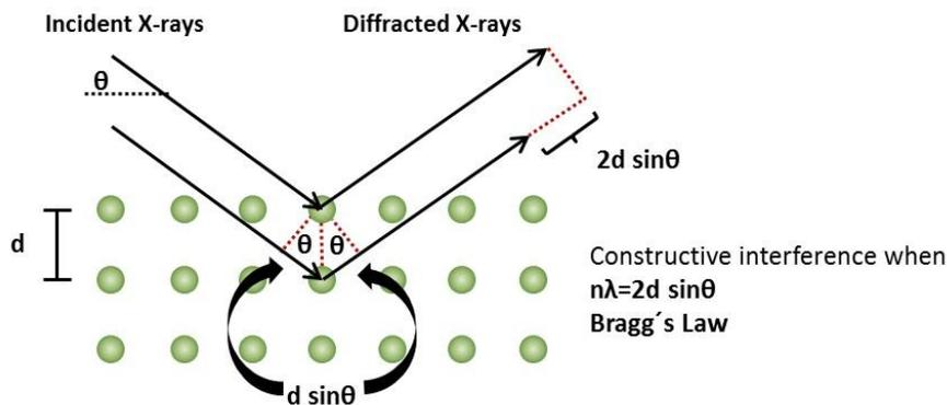
Figure 4. Schematic representation of the Bragg equation.
