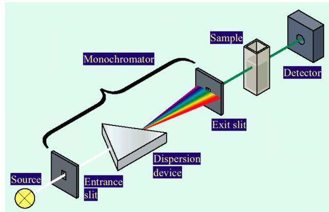
Figure 1 Scheme of operation of UV-Vis spectrophotometry. (Oliveira, A. & Araújo, M. 2011)
