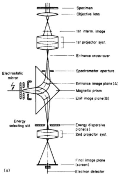
Figure 3. Beam path and optical configuration of the image electron energy loss spectrometer
