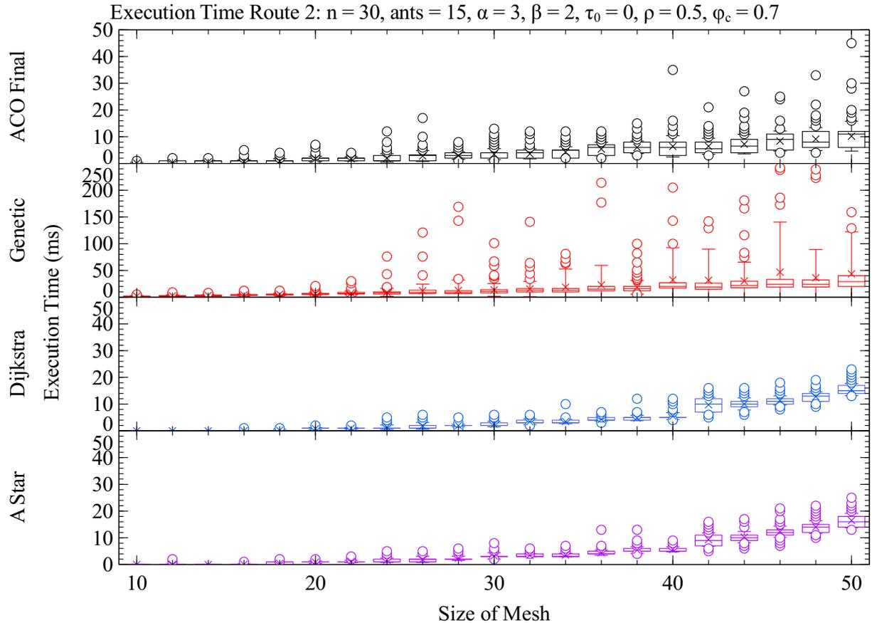
Figure 5.19: Route 2. Rerouting Time Comparison of Different Methods of Path Planning.
