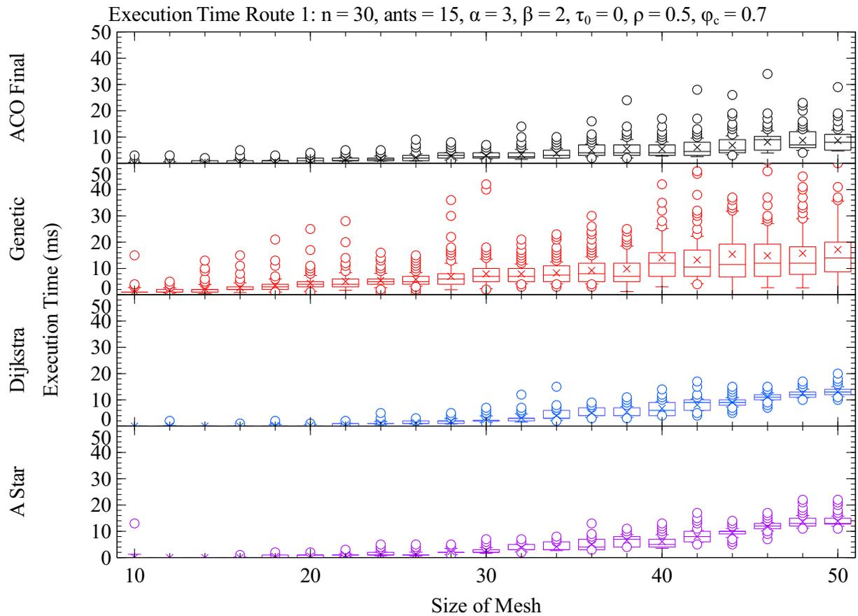
Figure 5.18: Route 1. Execution Time Comparison of Different Methods of Path Planning
