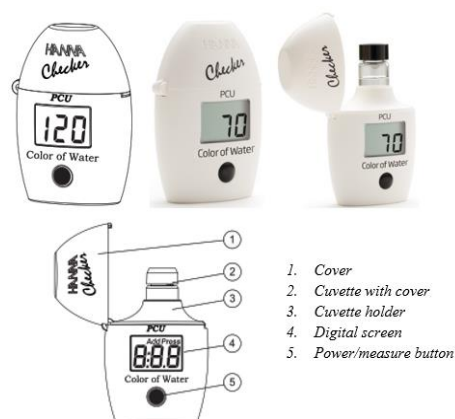
Figure 3.9. Illustration of the colorimeter checker (HI727 instrument provided by HANNA Instruments) proposed to evaluate the effectiveness of the filter design.
