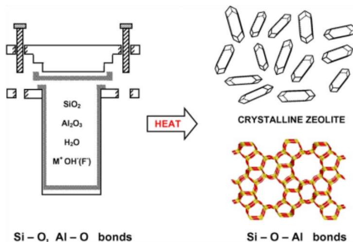
FIGURE 1.3: Hydrothermal zeolite synthesis. The starting materials are converted by an aqueous mineralising medium ( \text{OH}^- and/or \text{F}^- ) into the crystalline product whose microporosity is defined by the crystal structure [8].
