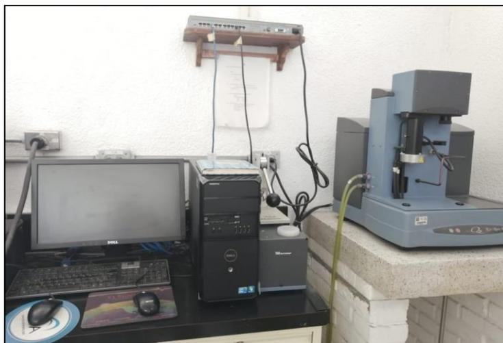
*Figure 15. TGA Q50 from TA Instruments USA*
