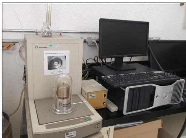
*Figure 16. Differential Scanning Calorimeter, TA Instruments*
