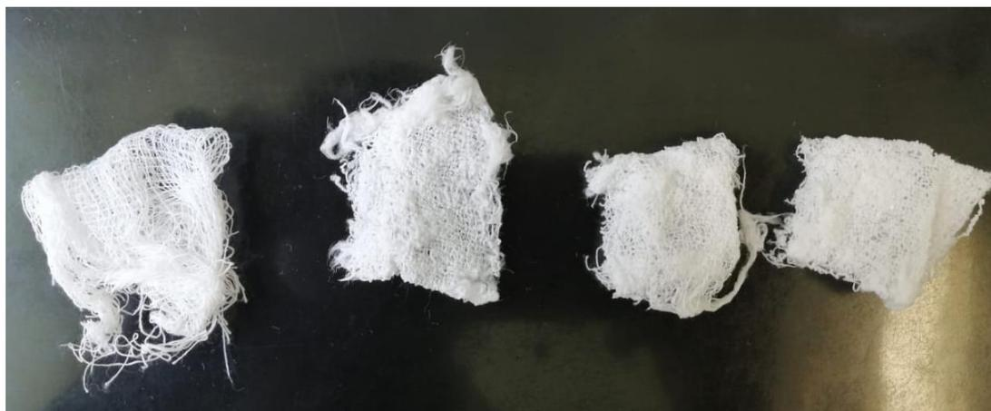
**Figure 22.** Pristine gauze, Gauze-g-MAAc (22%), Gauze-g-MAAc (74%), Gauze-g-MAAc (116%) (From left to right)
