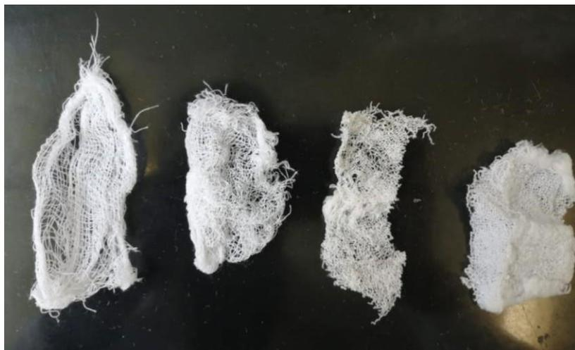
**Figure 21.** Pristine gauze, Gauze-g-AAc (26%), Gauze-g-AAc (52%), Gauze-g-AAc (143%) (From left to right)
