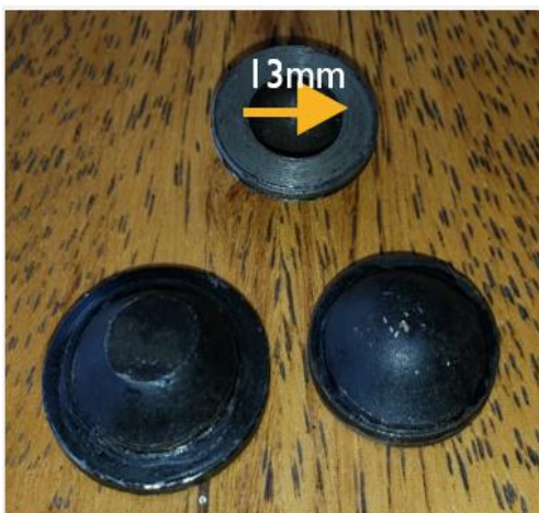
Figure 5: Spherical mold used for shaping the pellets 53 .
