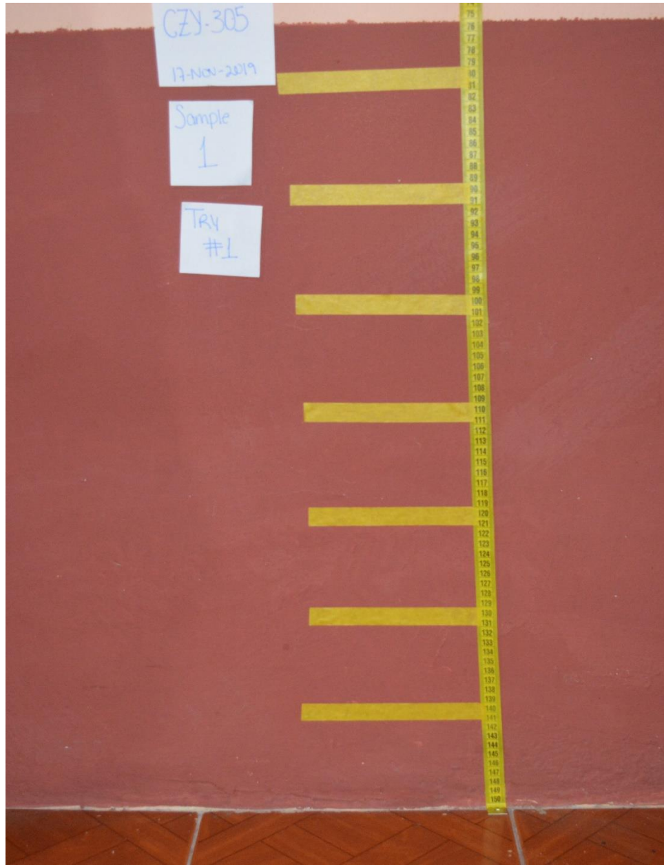
Figure 4 Free-fall drop test at 1.50m of height.
