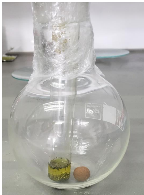
Figure 8 Assemble of FeS + HCl reaction with clay sample
