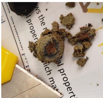
Figure 34 Clay after reactivity test, showing different color layers.
