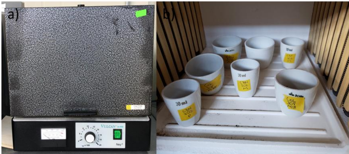
Figure 3 a) Muffle Vulcan A-550 b) Clay samples before calcination process.
