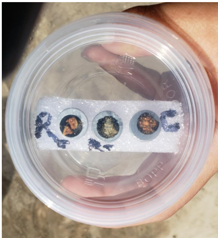
Figure 11 Raw, Reacted and Calcined (from left to right) clay of CZY-304 sample.
