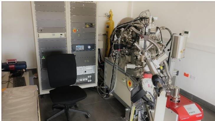
Figure 4.4: XPS equipment at Yachay Tech University used for measuring MWCNTs samples.
