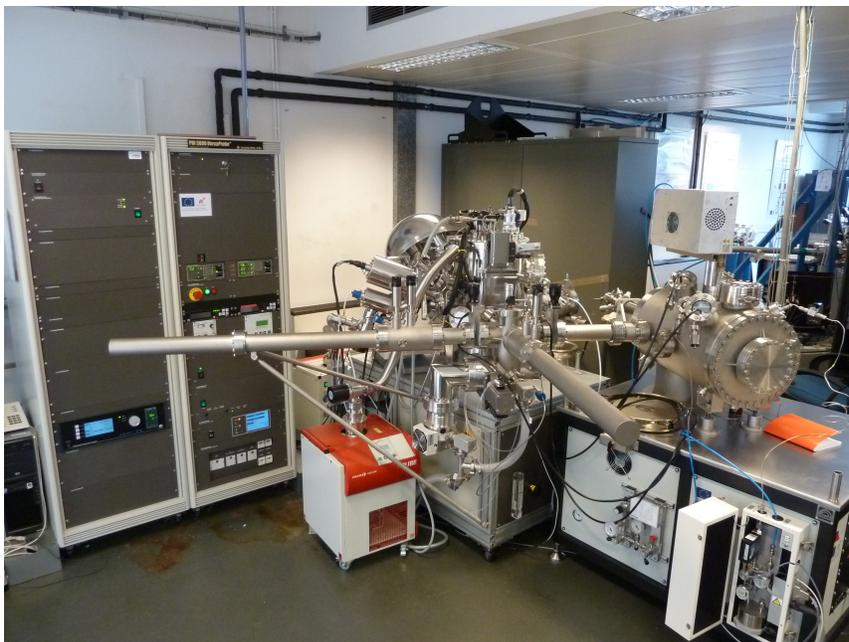
Figure 4.3: XPS equipment at MONS University used for measuring graphene samples.
