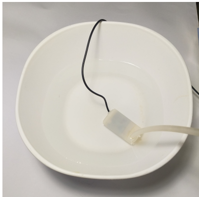
(a) Water Pump Connected to the Hoses
