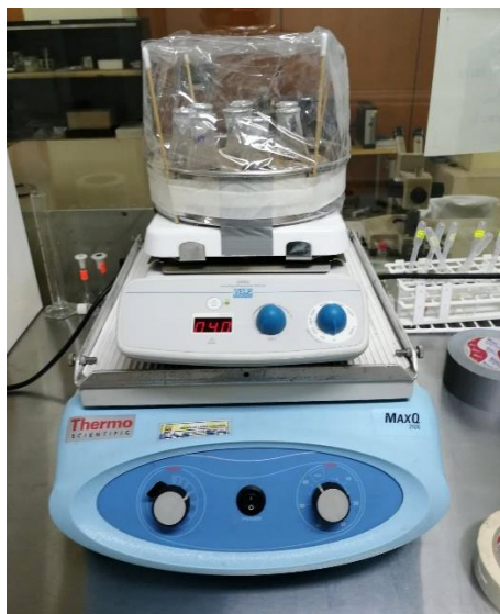
Figure 2: Adapted mechanism to incubate and agitate bacterial strains.
