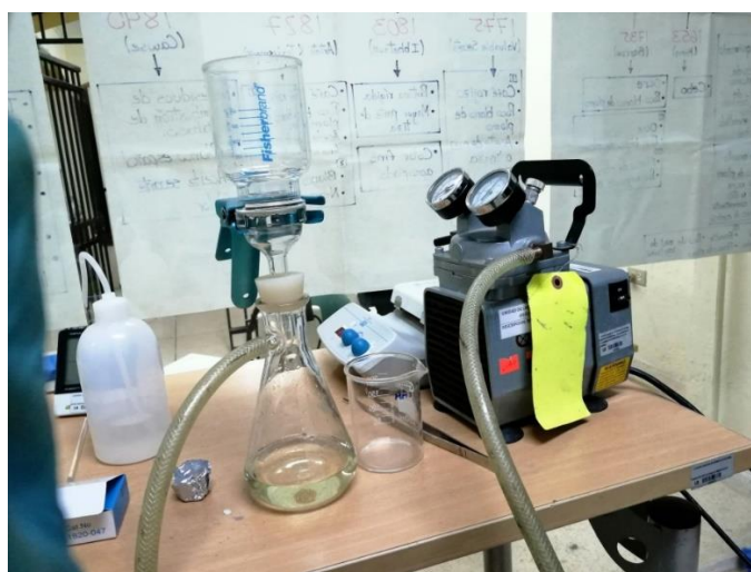
Figure 3: Vacuum filtration setup
