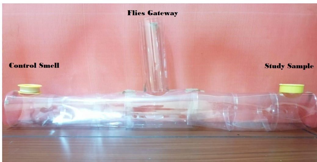
Figure 7. Prototype for analysis of simuliids preferences. The control smell is a neutral smell known to not elicit any particular response by the black flies.
