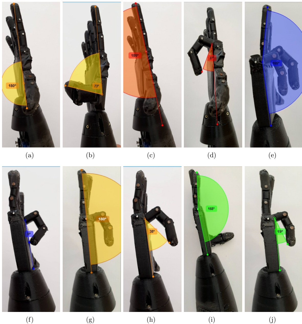
Figure 5.10: Angles of movement of each finger of the prosthesis: (a) thumb finger extended, (b) thumb finger flexed, (c) index finger extended, (d) index finger flexed, (e) middle finger extended, (f) middle finger flexed, (g) ring finger extended, (h) ring finger flexed, (i) little finger extended, (j) little finger flexed.
