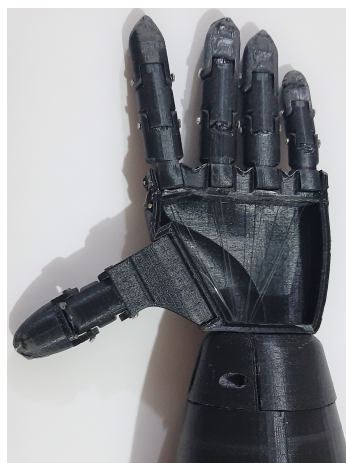
Figure 5.6: Parts of the fingers connected with nylon thread and use of nails for the joints.
