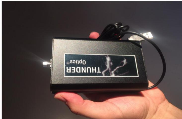
Figure 3.7: SMA Mini spectrometer manufactured by Thunder optics. Source: Reprinted from SMA Mini Spectrometer » Thunder Optics<sup>6</sup>
