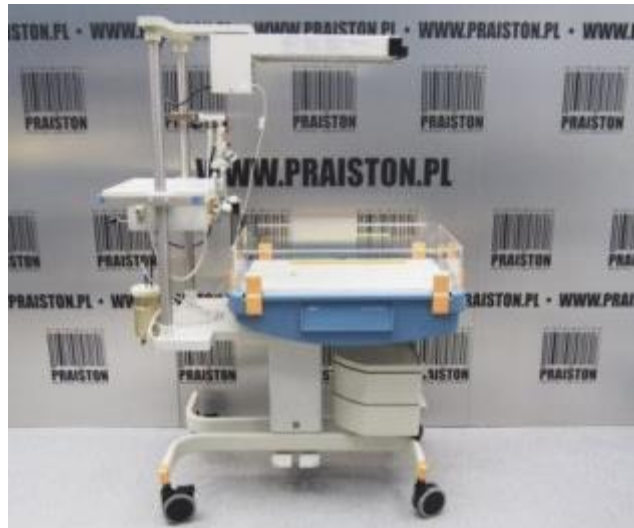
Figure 4. Open box neonatal incubator. Source: https://www.machinio.com/listings/38050615-open-incubator-drager-babytherm-8000-resuscitation-station-in-leszno-poland
