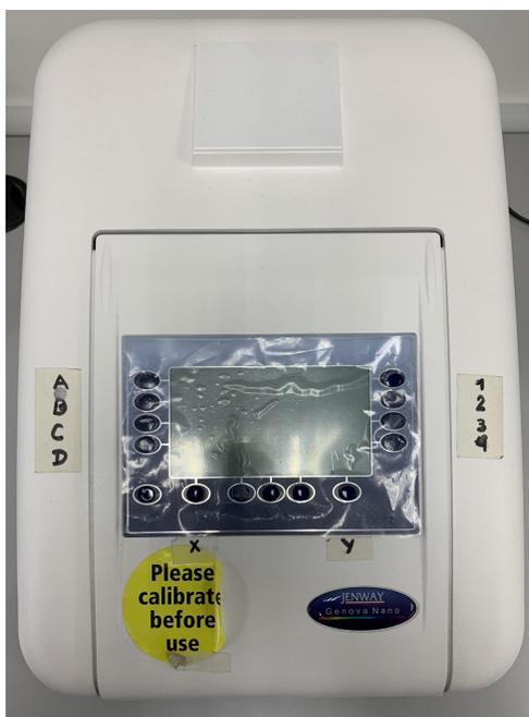
Figure 5.4: UV-vis spectrometer JENWAY Genova Nano.
