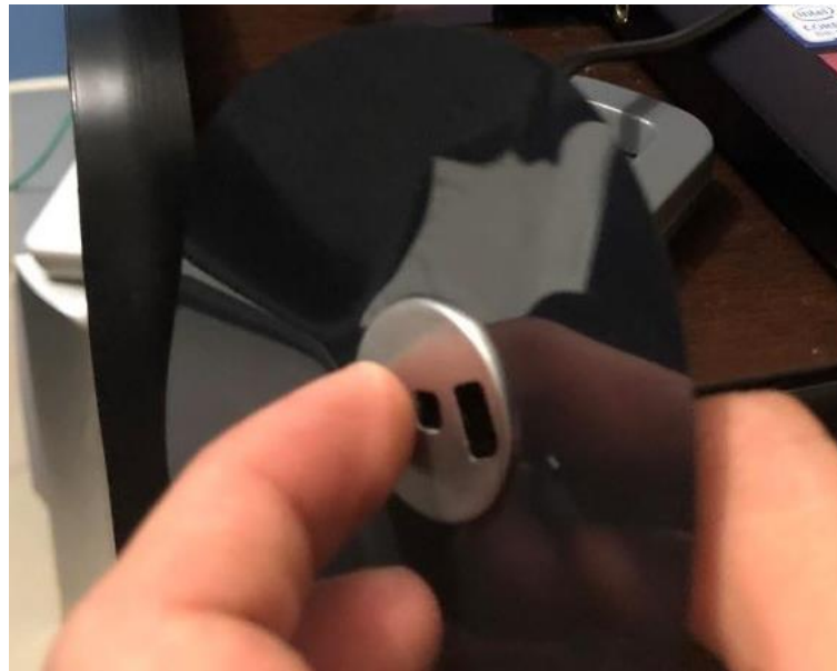
Figure 16. Internal part of the floppy disk used as a visible light filter in the early phases of the project.
