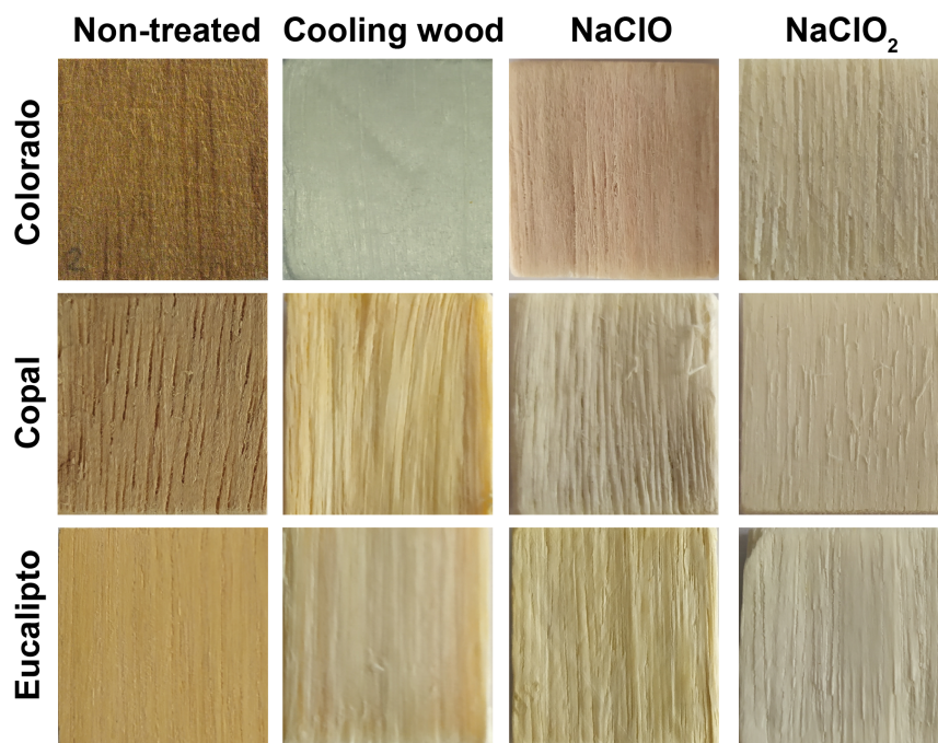
Figure 4.1: In this figure one observes the materials obtained from Colorado, Copal and Eucalipto woods, after chemical treatment with NaOH/Na 2 SO 3 and H 2 O 2 (cooling wood), NaClO and NaClO 2 .
