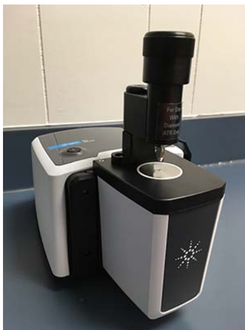
Figure 5.5: FTIR Spectrometer - Agilent Cary belonging to Yachay Tech University, Ecuador.
