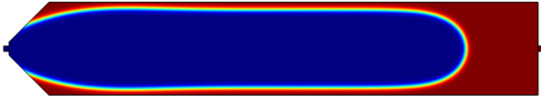
Figure D.2: Simulation of finger structure at b=3\text{mm} , plot case d. The blue region is the portion of water in the displacement, the red region is the oil displaced.
