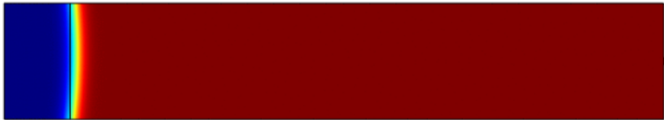
Figure 6.8: Flat interface geometry. The blue portion corresponds to water, the red portion is oil. The flow goes from left to right.
