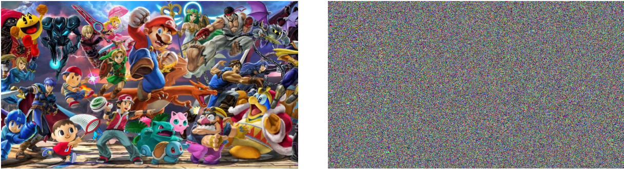
Figure 4.8: Left: Original .jpg color image. Right: Decoded image with a small difference in initial conditions. The original image was codified with initial conditions \mathbf{x}_0 = (10.0, 10.1) and decoded with \mathbf{x}_0 = (10.0000000000001, 10.1) . CMN fixed parameters are: \mu = 1.4 , z = -0.25 , \epsilon = -0.025 .
