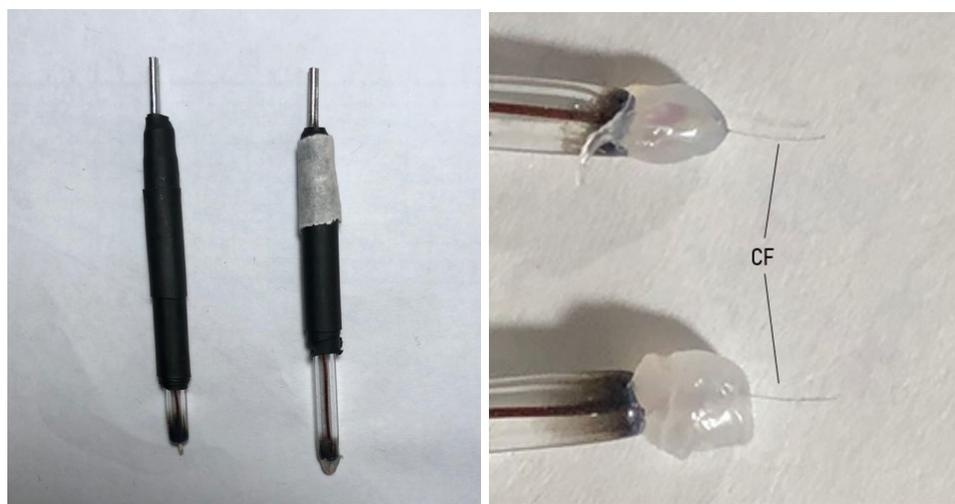
Figure 3.16: Left hand side:Electrodes for attaching CFs. Right hand side: Fibers attached to the electrode tip.
