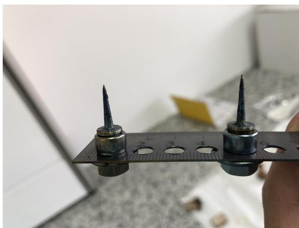
Figure 3.3: Spike mounting for pyrolyzing fibers inside the tubular furnace.
