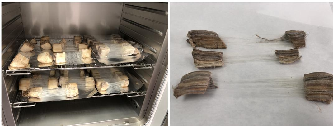
Figure 3.7: LHS: Fibers left into the oven at 65 °C. RHS: Dried fibers ready to pyrolyze.
