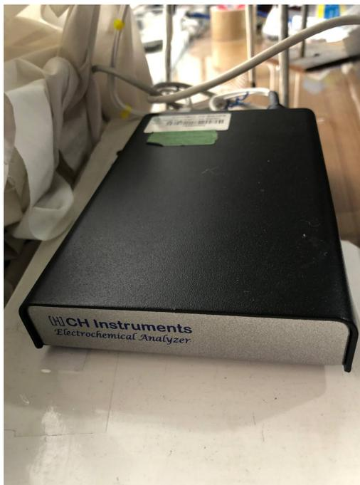
Figure 3.22: Potentiostat, CH Electrochemical Analyzer.
