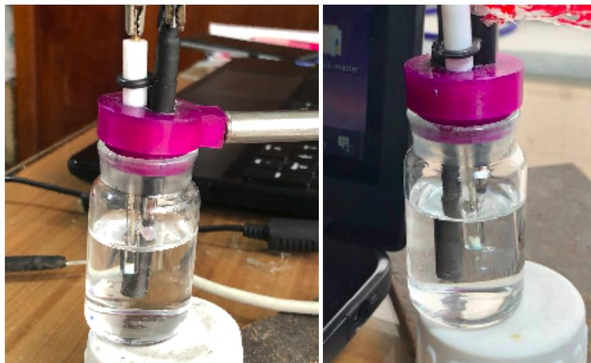
Figure 3.38: Cell design for CV.
