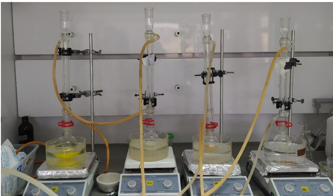
Figure 17 Experimental set up for the synthesis of ligands and complexes
