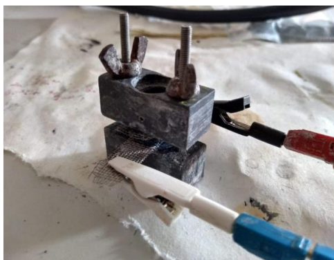
Figure 8 Zn / GPE / Zn configuration cell used for CV.
