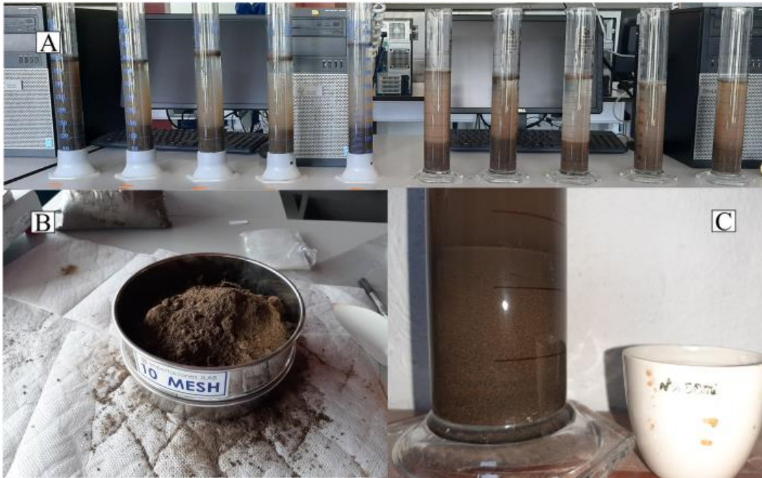
Figure 11. Process for obtaining the texture of the soil. [A]. Samples sedimented into the test tubes after 20 hours. [B]. 2-mm sieve with sample to be sifted. [C]. Formation of horizons with the different sizes of the particles by the density of each of its.
