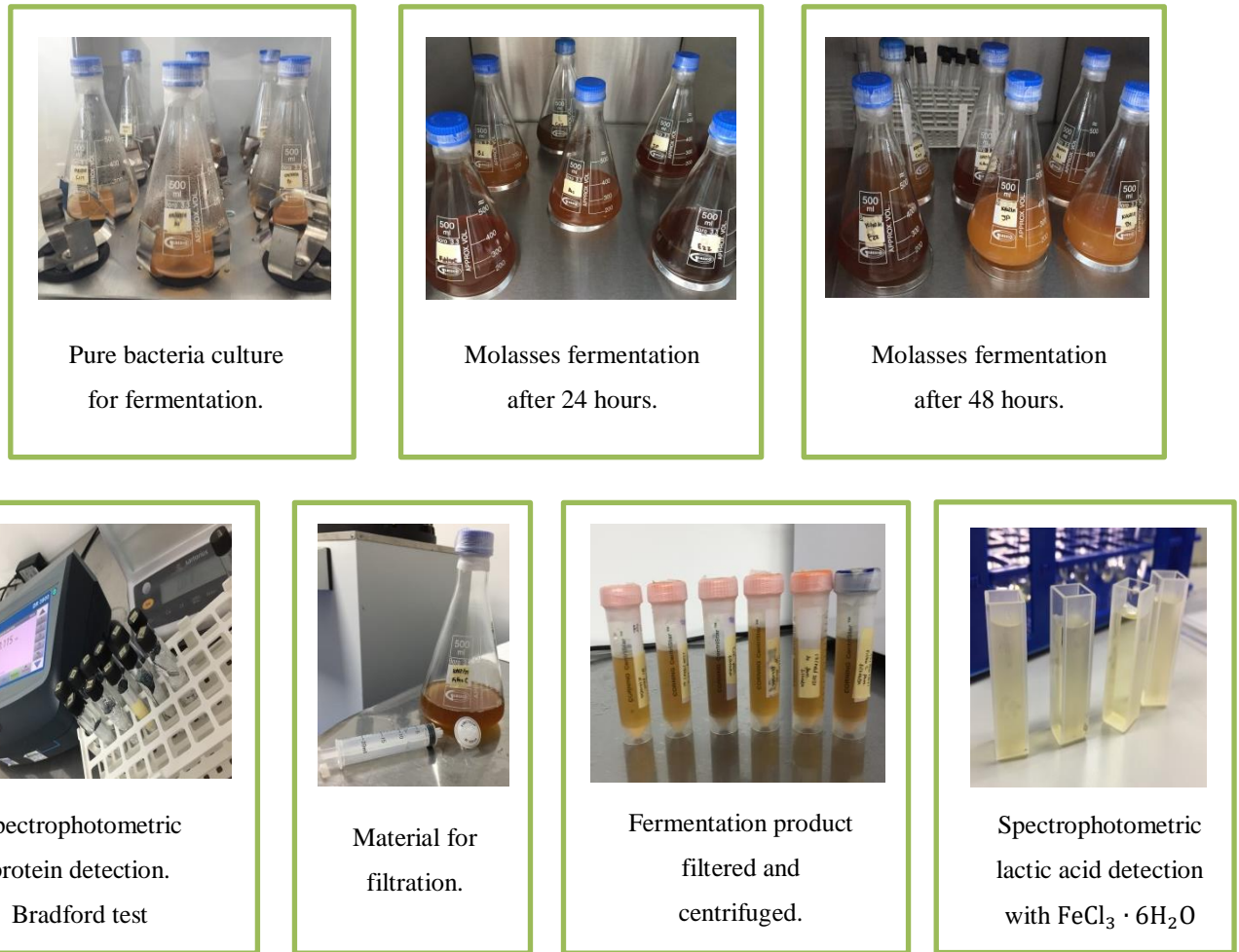
Figure 4. Scheme of the proposed preliminary molasses fermentation. This scheme is to perform the preliminary study for the bacterial industrial potential in terms of protein and lactic acid production.
