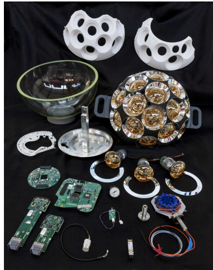
Figure 2.2: Internal Components of the KM3NeT DOM. All the readout, control system, and power supply are managed by the CLB.
