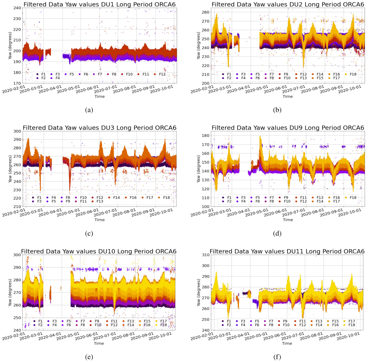
Figure 4.4: Reconstructed Yaw (Y) values for ORCA6 compasses in Long-Period (includes Short-Period). Each color represents compass readouts along the DU. Time format: yyyy-mm-dd.
