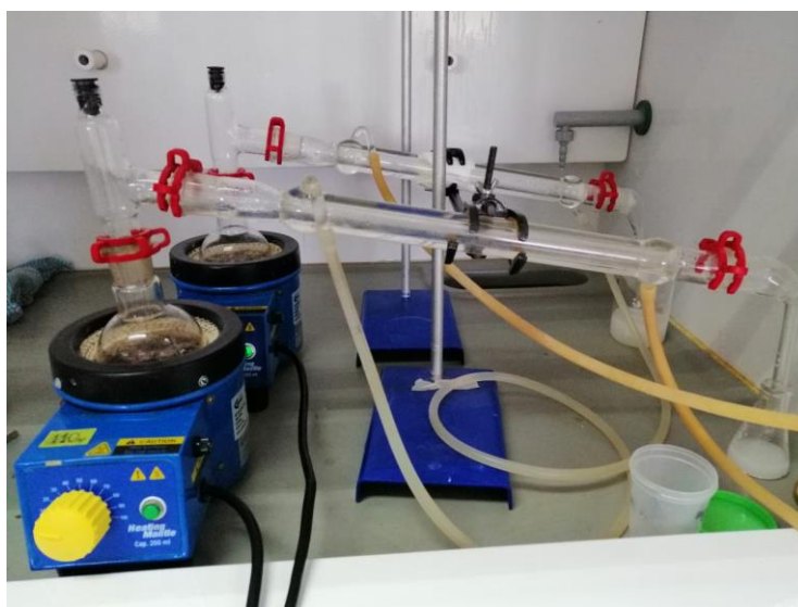
Figure 6. Simple distillation system used in the extraction of cinnamaldehyde.
