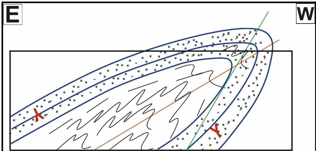
Figure 23. Schematic picture of the recumbent fold of the Chota Fm. The rectangle represents the outcrop seen in the field. The blue lines represent the sandstone sequences with its respective polarity symbol in red. The central part of the fold is completely deformed and with the presence of small-scale chevron folds. The red line indicates the axial plane. The green line represents a large-scale fault that cuts the outcrop.
