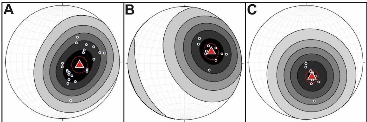
Figure 29. A) Stereonet representation of the joint's measurements in The Chota Fm (n=22). B) Stereonet representation of the joints that dip to the west in Chota Fm. C) Stereonet representation of
