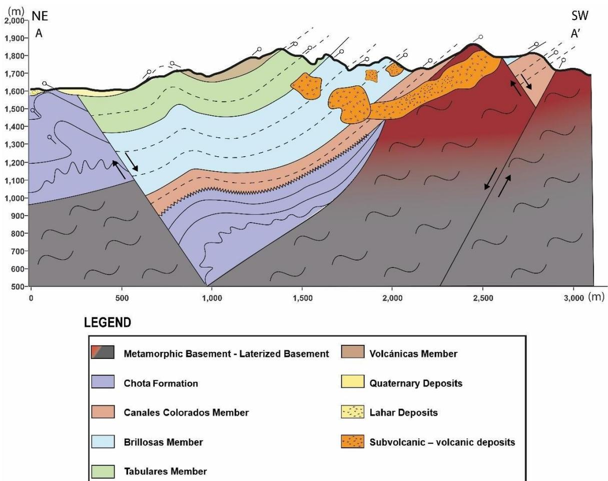
Figure 30. Structural Cross section of the study area. The location of the profile can be seen in Figure 6.
