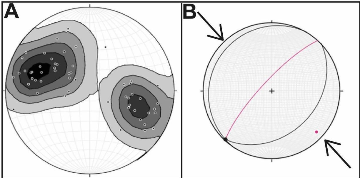
Figure 25. A) Stereonets of the chevron folds of the Chota Fm (n=30). Contours obtained with the Kamb method (Kamb, 1959), with 2 sigma contour intervals. C) Stereonet of the planes to the fold, the pink line is the axial plane of the folds, and the pink point is the pole to the axial plane, that represents the mean direction of the stress = 11°/132°; the black point is the hinge line.
