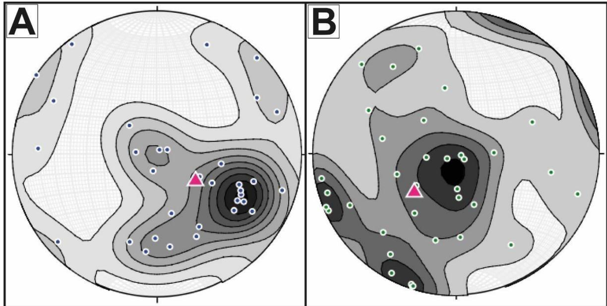
Figure 21. A) Stereonet of fold test of the faults of the Chota Fm B) Stereonet of fold test of the faults of the Peñas Coloradas Fm. Blue points are the poles of the Chota faults. The green points are the poles of the Peñas Coloradas Fm faults. The pink triangles represent the Fisher mean vector. Contours obtained with the Kamb method (Kamb, 1959), with 1 sigma contour intervals. All stereonet are plotted on a lower hemisphere, equal-area stereonet projection.
