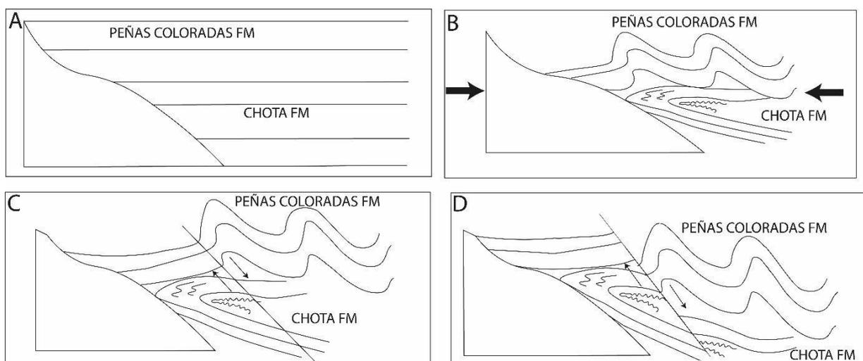
Figure 33. Schematic representation of the second evolution model of the study area. A) Stage 2. B) Stage 3, the arrows represent the compression that modelate the folds of the study area. C) Stage 4.
