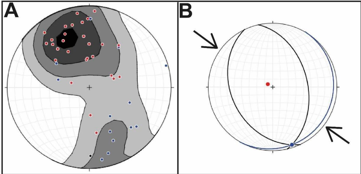
Figure 24. A) Stereonet of Fold C. of the Chota Fm (n=42), representation of the poles; the red points are the poles of the upright limbs of the fold; the blue points are the poles of the overturned limbs of the fold. Contours obtained with the Kamb method (Kamb, 1959), with 2 sigma contour intervals. B) Representation of the axial plane of the fold (blue line), and the pole of this axial plane (red point); the blue point is the hinge line of the fold. The arrows indicate the  $\sigma_{Hmax}$ .
