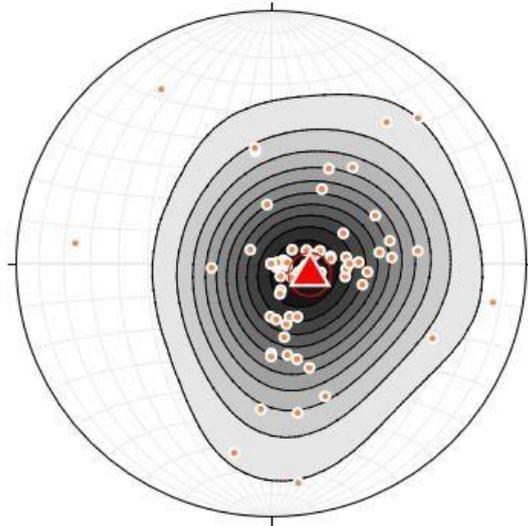
Figure 28. Stereonet representation of the joint's measurements in Peñas Coloradas Fm (n=68). The triangle represents the mean vector. Contours obtained with the Kamb method (Kamb, 1959), with 3 sigma contour intervals.
