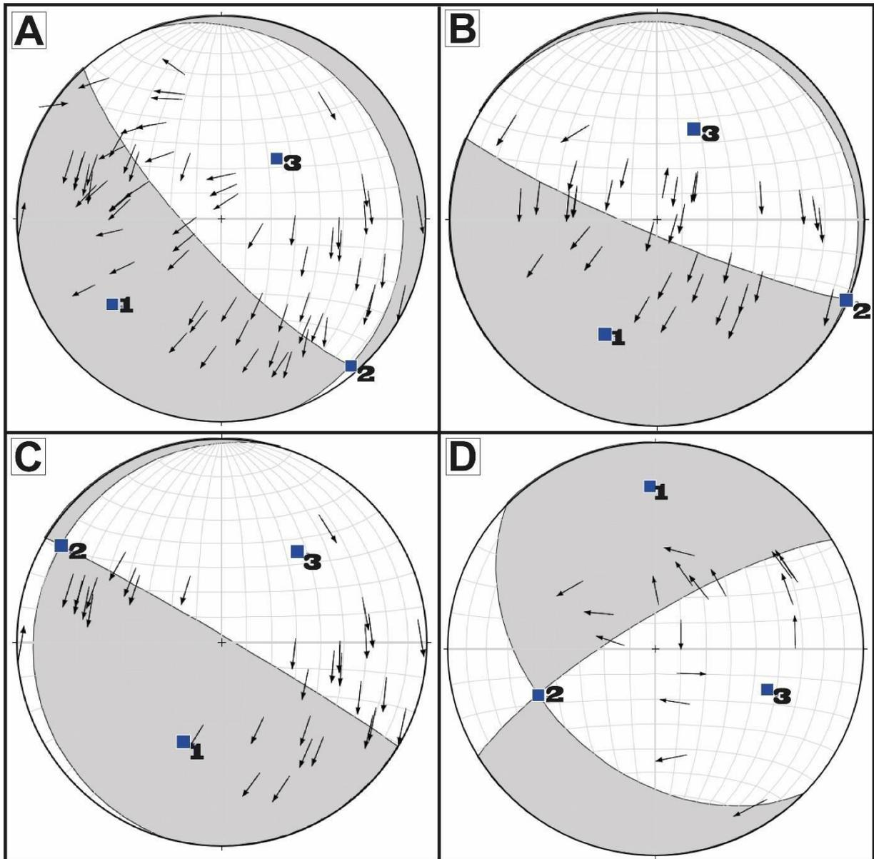
Figure 22. A) Stress inversion results obtained from 68 faults. B) Faultkin results obtained from the Peñas Coloradas Fm faults (n=35). C) Faultkin results obtained from the Chota Fm faults (n=33). These are Fault plane solutions, the blue squares and numbers represent the orientations of the principal stresses where P = 3, and T=1. The arrows show the tangent lineations of each measurement.
