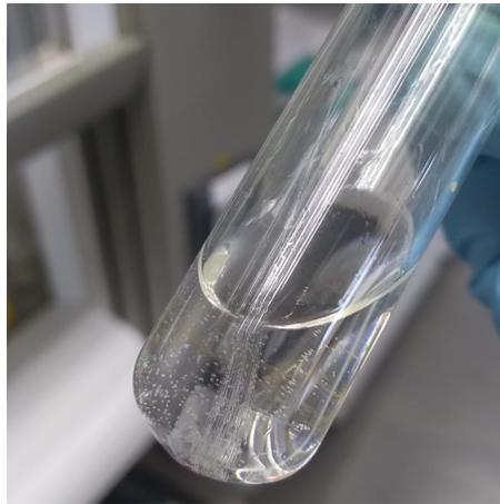
Figure 3.4: Optical fibers immersed in piranha solution for removal of organic material.
