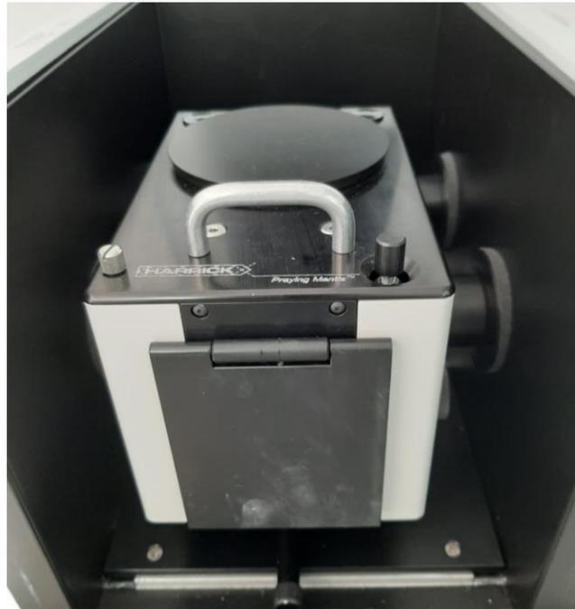
**Figure 2.6** Accessory used for DRS.
