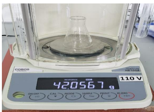
Figure 14. Weight of the Erlenmeyer flasks before introducing the pellet formed from the samples.
