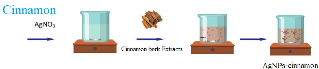
Figure 9 Scheme of Green Synthesis of AgNPs using cinnamon as reducing agent
