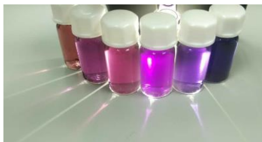
Figure 16 Tyndall effect scattering of AgNPs-H.
