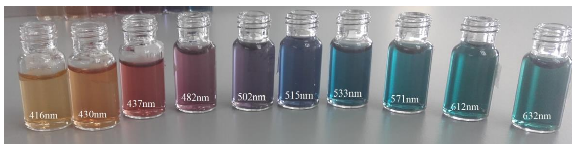
Figure 23 Spectra from UV-VIS spectroscopy of the SPR phenomenon of the different AgNPs-Hydrazine obtained using different volumes of silver nitrate 1 mM indicated in the inset of the figure.
