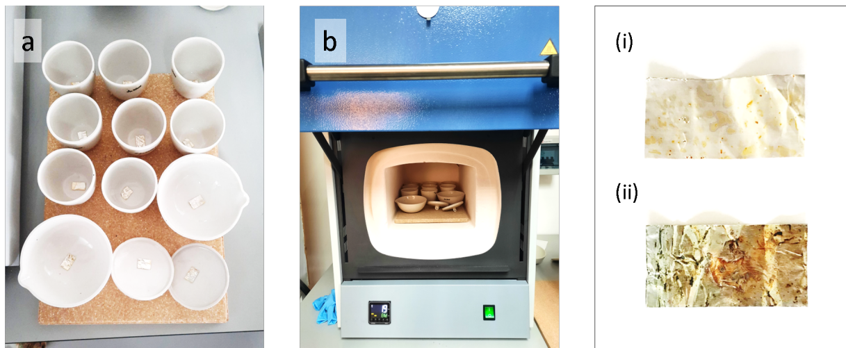
Figure 3.6: Calcination process of the sa-Al substrates loaded with the catalyst solution; (a) inside melting pots, (b) melting pots with sa-Al inside the muffle furnace, and sa-Al substrate (i) before and (ii) after the calcination.
