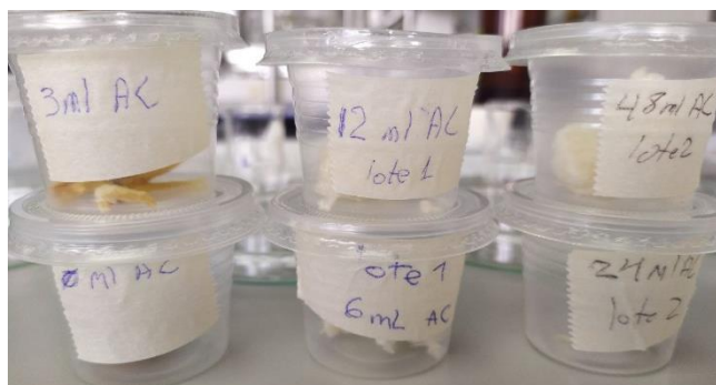
Figure 17. Hydrogels materials at different concentrations of Citric Acid.
