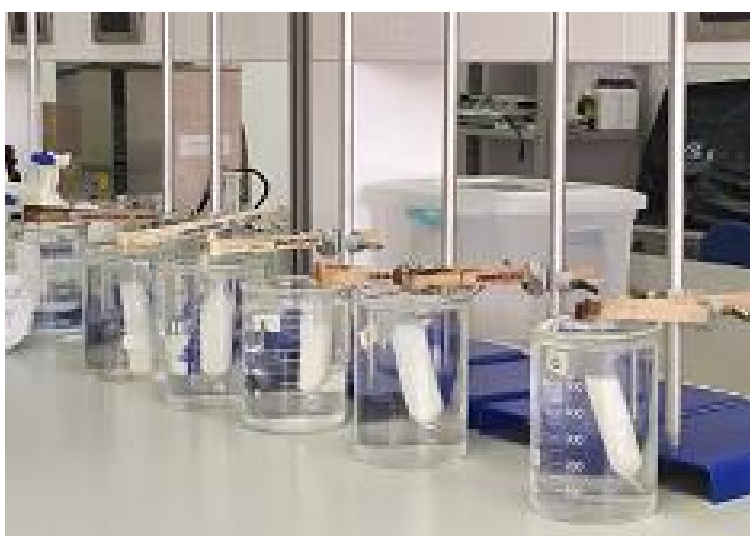
Figure 5-2. Dialysis System to cellulose from OPEFB
