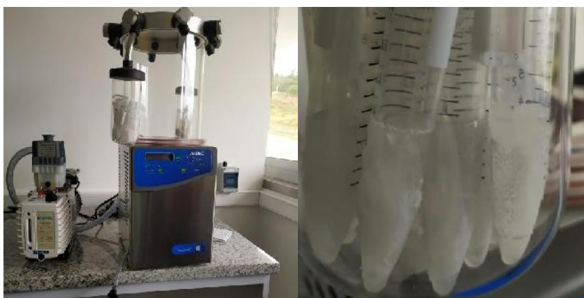
Figure 5-3. Freeze-drying process on CNC from OPEFB
