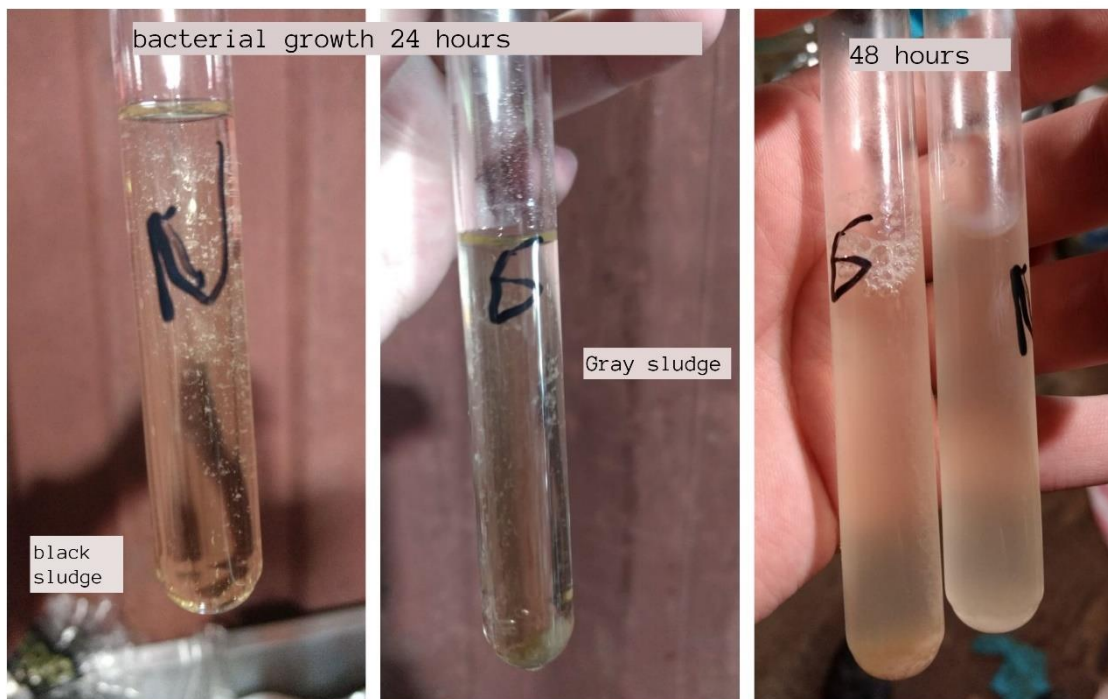
Figure 6: Bacterial growth in test tubes with gray water sludge and black water sludge at 24 and 48 hours. The analysis of these samples was qualitative to observe only the type of bacteria that grew in the tubes.
