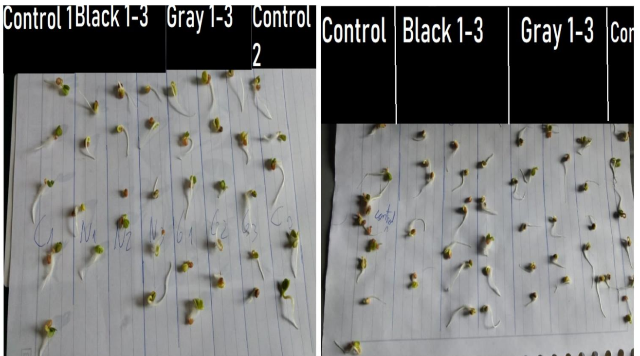
Figure 2: Germination of radish seeds exposed for 72 hours to black and gray water sludge from the “X camp”. The seeds exposed to black water mud presented short roots or a remarkable inhibition of the germination stages in all the repetitions. In the case of the seeds exposed to gray water mud, they showed long and very thin roots. Finally, the control allowed to compare the process of inhibition and abnormalities of the seeds when germinating with WWTP sludge.
