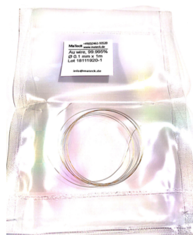
Figure 3.1: Gold metal wire for the construction of the electrodes with an ultra-high purity of 99.999%.
