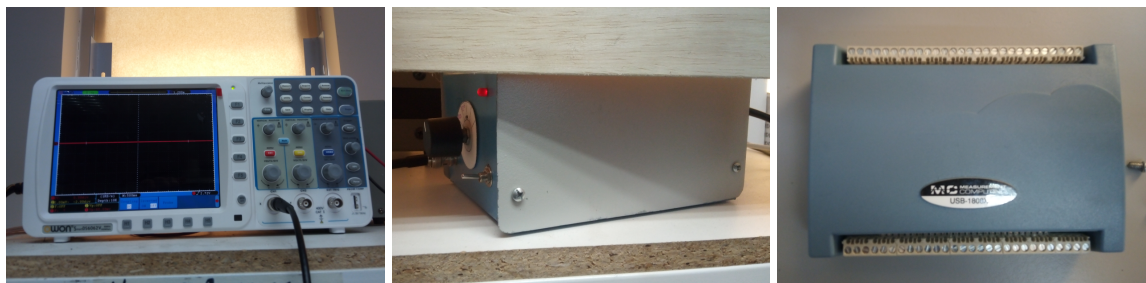
Figure 3.5: Fast electronics equipment. Left: Oscilloscope. Center: I/V preamplifier, in this experiment for metallic junction amplifies the signal 10^5 and for molecules 10^6 . Right: DAQ from Measurement Computing, model USB-1808X, with a resolution of 18 bits and a max sample rate of 200 KS/s .
